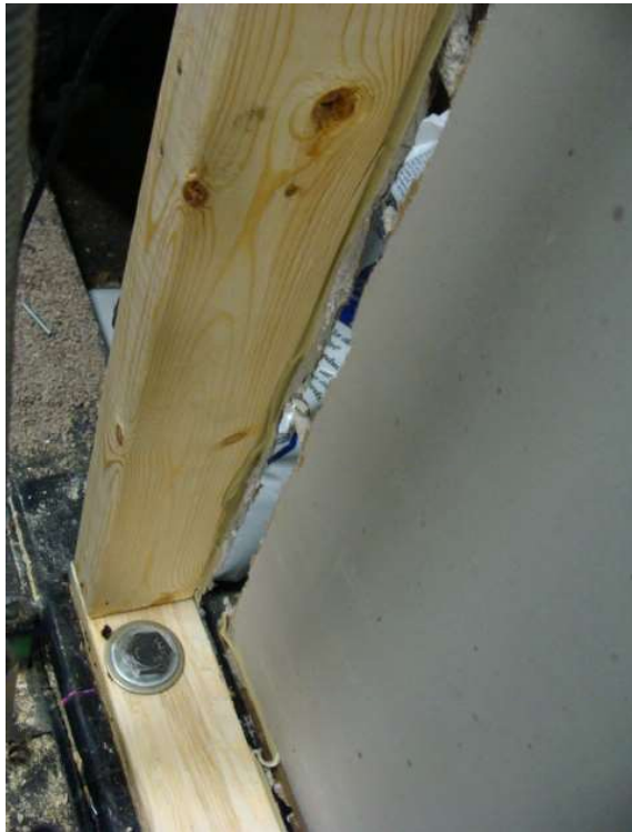
Photo 9: Typical Failure- Drywall Shear
