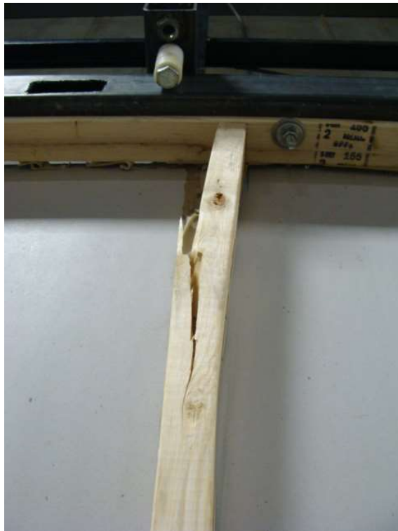
Photo 9: Typical Failure- Drywall Shear
