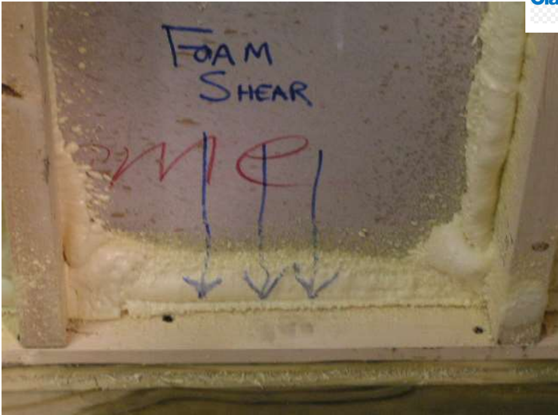
Test #3 bottom plate failure
